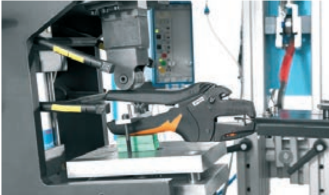
Testing the endurance of stripax® in the Weidmüller laboratory
